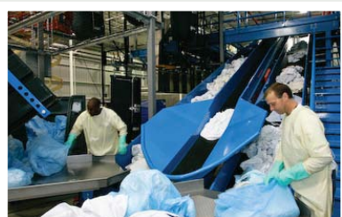
▶ Soil sort conveyor.
