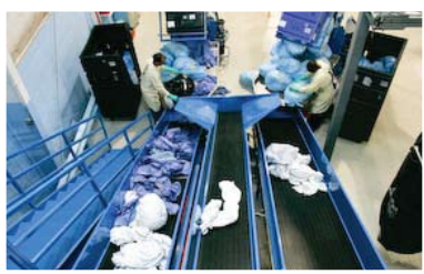
▶ Top view of soil sort conveyor.
